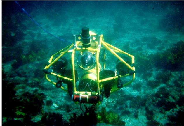
**Figure 10.4** Underwater vehicle Oberon, developed at the University of Sydney. Image courtesy of Stefan Williams and Hugh Durrant-Whyte from the Australian Centre for Field Robotics, University of Sydney, Australia.
